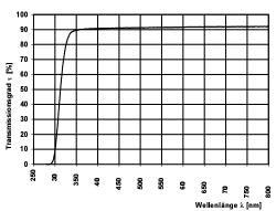
The light transmittance for a thickness of 0.15 mm is  $\tau_{VD65}$  in % (d=0,15 mm) = 91,7  $\pm$  0,3%. In the visible range of the spectrum D 263 M is without absorption. The excellent UV absorption properties makes D 263 M an ideal material for use in fluorescence microscopy.
